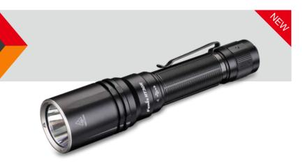
Fenix HT30R is a white laser tactical flashlight with an ultra-long beam of 1500 meters. The light neck has a hidden Type-C charging interface, powered by a single 21700 high-capacity Li-ion battery. The dual tail switch activates instant on and strobe function. It can quickly respond to operations in military and law enforcement, personal hunting, emergency rescue, personal defense and other activities.
